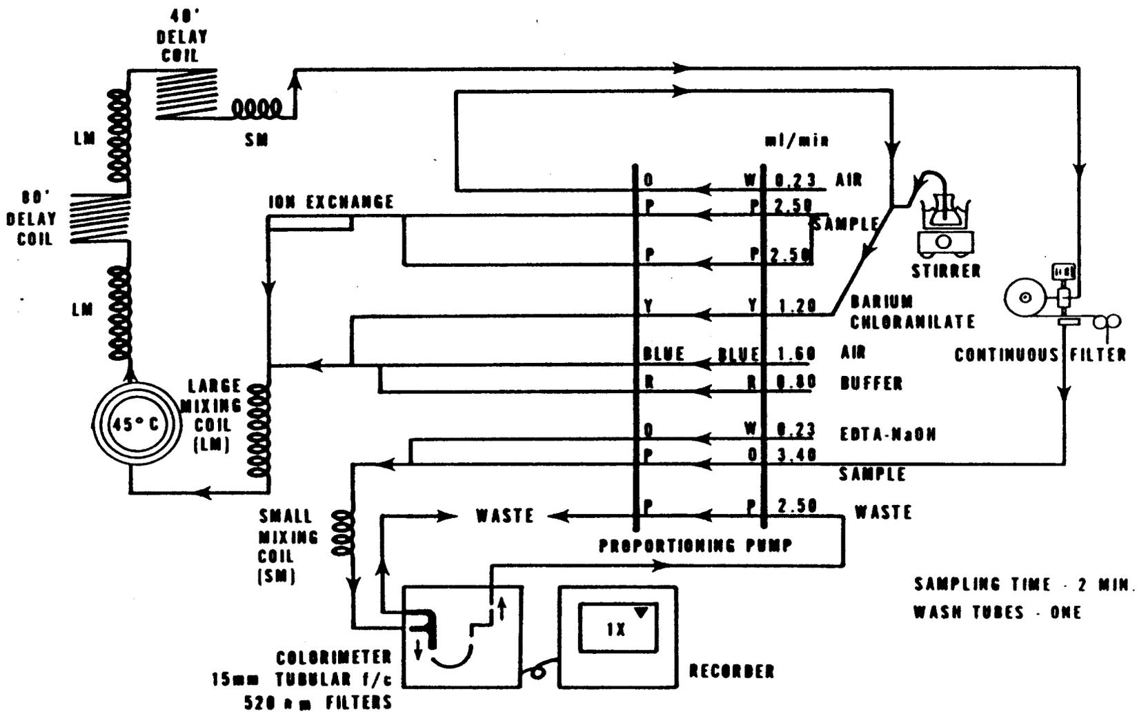
FIGURE 1 - SULFATE MANIFOLD AA-1
